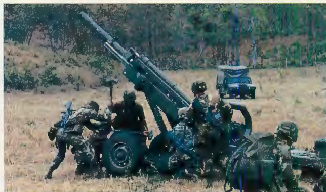
BELOW: M102 being laid in. Note roll bar across the breech and sight area of the howitzer, installed by the 82nd for protection in the event cross winds catch the chute and roll the gun over after a paradrop.
